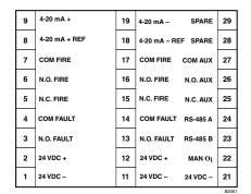
Wiring Terminal Identification for Standard X5200
